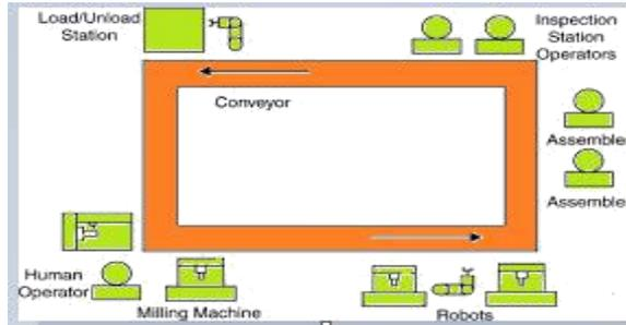
Figure-BLOCK DIAGRAM OF FLEXIBLE MANUFACTURING SYSTEM
